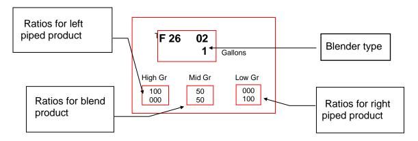
1) In mode 26 on the right side of the gallon display window a **0**,**1 or 2** may be showing in the gallon window. This option sets the *Blender type.*
