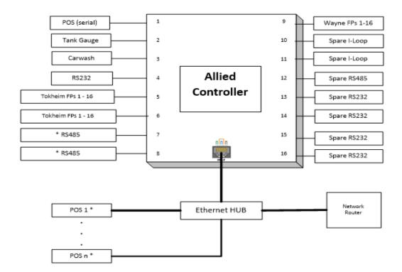
This figure describes the Allied Controller to a Tokheim-Wayne system installation. \* Note: denotes alternative POS connectivity options (RS232 vs. Ethernet)
