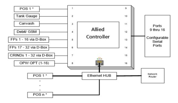
This figure describes the Allied Controller to a Gilbarco system installation with the OPT. For Windows connectivity on Aegis controller, refer to the Aegis User Manual.
