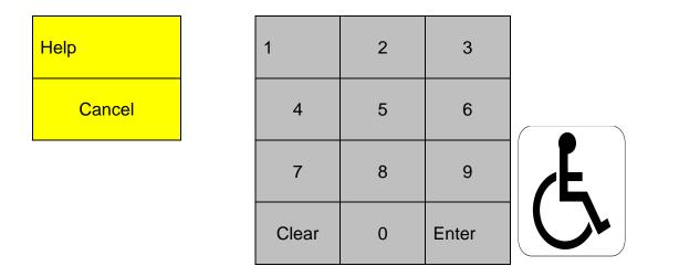
Note: This type 5 and 6 keypad configuration will support the location of the Help, Cancel and ADA buttons on either side of the numeric keypad.
