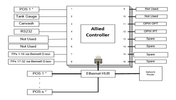
This figure describes the Allied Controller to Bennett system installation with the OPT and the IPT. \* Note: denotes alternative POS connectivity options (RS232 vs. Ethernet)
