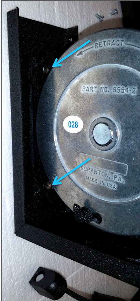
Figure 13. enclosure bracket with 2 pre-drilled holes for mounting
