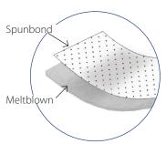
One layer of spunbond fabric is bonded to a single layer of meltblown polypropylene.
