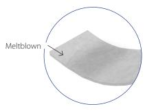
Single layer of standard fiber meltblown polypropylene.
